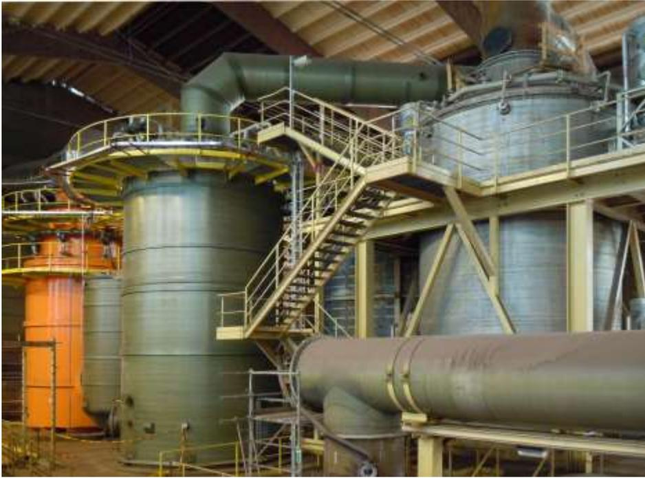
Pic. 6: Complex multistage wet scrubbing unit installed at a metallurgical plant.
